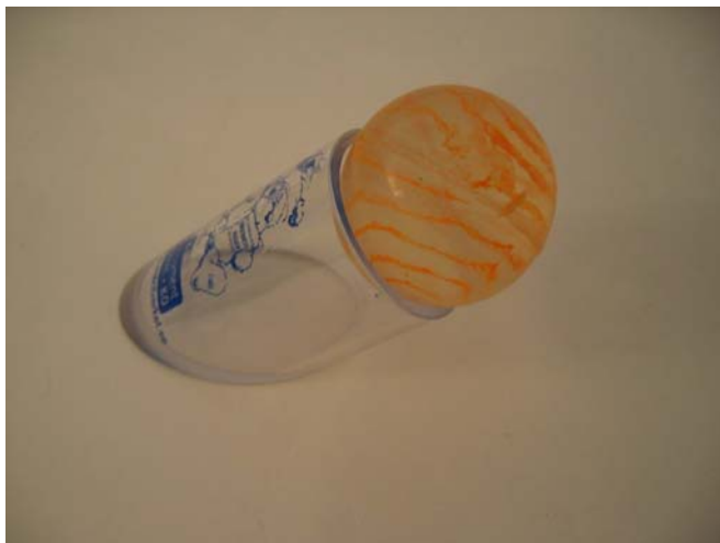
Figure 4 Round ball that does not fit in the 32 mm diameter test cylinder.
