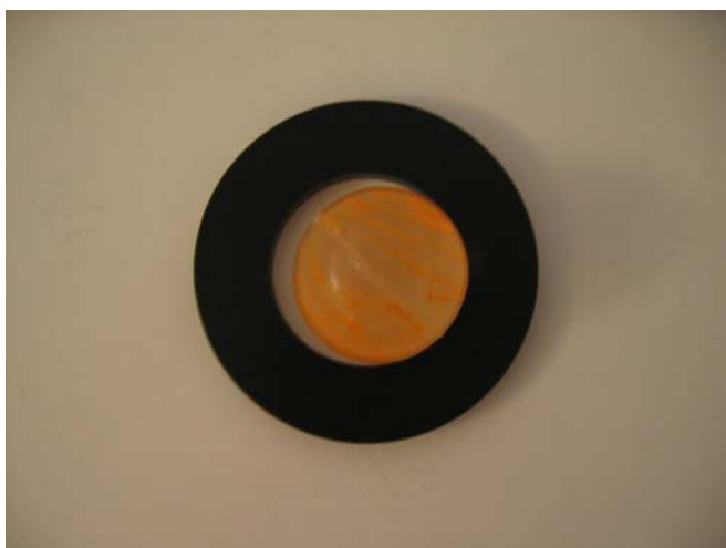
Figure 5 Round ball that passes through the 44.5 mm diameter template E
